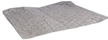
Single meltblown core sandwiched between nylon skins and perforated.
